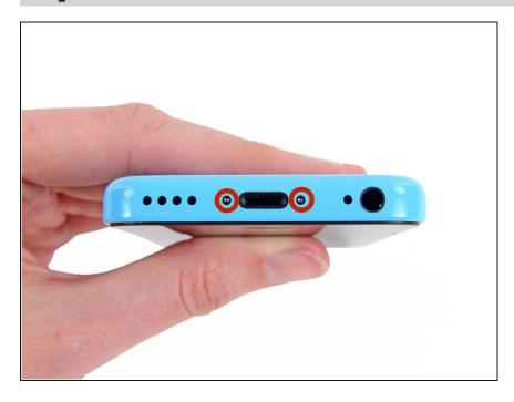
Use the Pentalobe screwdriver to remove the two 3.8 mm Pentalobe screws near the dock connector.
