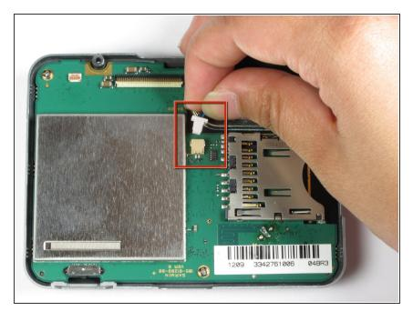
Pull the cable out to detach the speaker from the logic board.
