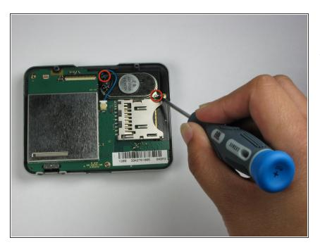
Unscrew the two screws on opposite sides of the speaker using the #00 Phillips screwdriver.
