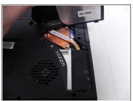
Remove the cover from the cooling unit.
