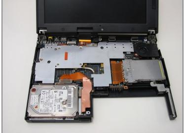
• Carefully lift and remove the keyboard.
