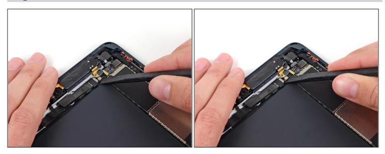
• Use the flat end of a spudger to pry the top right antenna's coaxial connector from its socket on the logic board.
