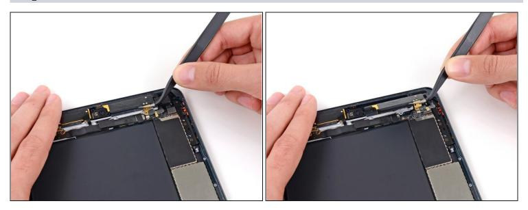
• Use tweezers to lift and remove the top right antenna from the rear case.
