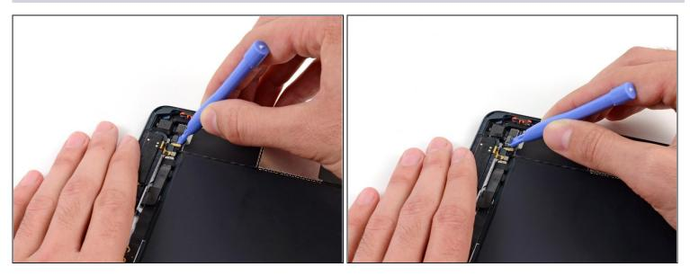
• Use a plastic opening tool to pry the top right antenna ribbon cable up from its socket on the logic board.
