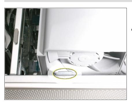
Replacement Note: Also make sure the latch on the inside top left edge of the fan assembly engages with the slot on the inside lip of the enclosure To reassemble your device, follow these instructions in reverse order.
