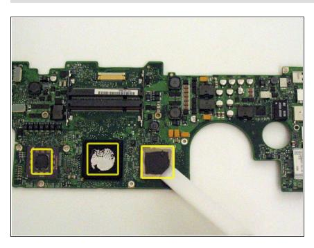
Use a firm plastic edge to scrape the thermal material off the three indicated chips.
