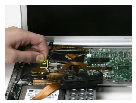
Disconnect the black and white RJ-11 cable from the top, right corner of the modem.
