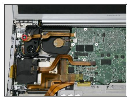
Remove the single T8 Torx screw from the left speaker assembly.
