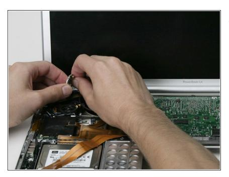
Lift the Bluetooth board partially out of the computer and disconnect the attached antenna cable.
