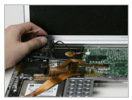
Deroute the cables from the right side of the speaker and lift it off of the logic board.
