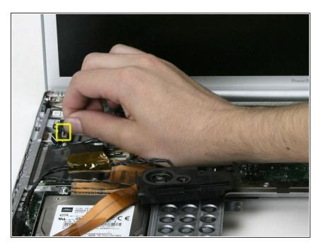
Disconnect the rainbow power cable from the DC-In board.
