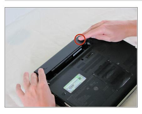
On the opposite side of the battery, press the release latch and slide the battery away from the main body to remove.
