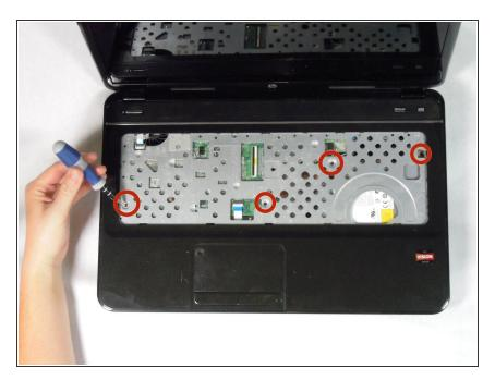
Unscrew the four 7 mm Phillips #1 screws on the board.
