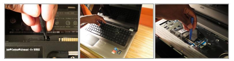
To the left of the battery connector is a keyboard release latch. Use a spudger to release the keyboard.
