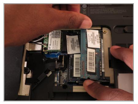
• Remove RAM by pushing the locking clips outwards.
