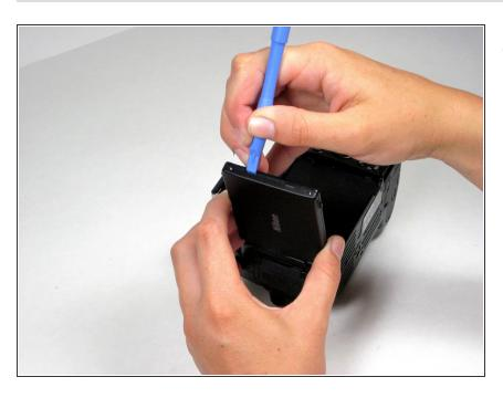
Using a fingernail or the flat edge of a spudger inserted into the seam, separate the LCD bevel from the main panel body.
