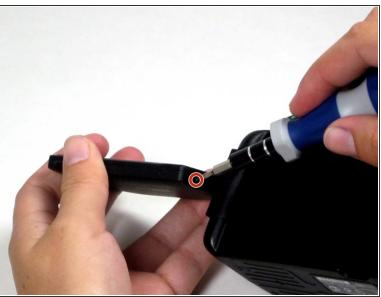
Use a Phillips #000 screwdriver to remove the four screws around the perimeter of the LCD panel.
