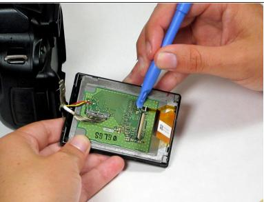
Use a spudger to remove the ribbon cables on the LCD's circuit board by flipping up their plastic lock-bars and removing gently pulling them out of their ports.
