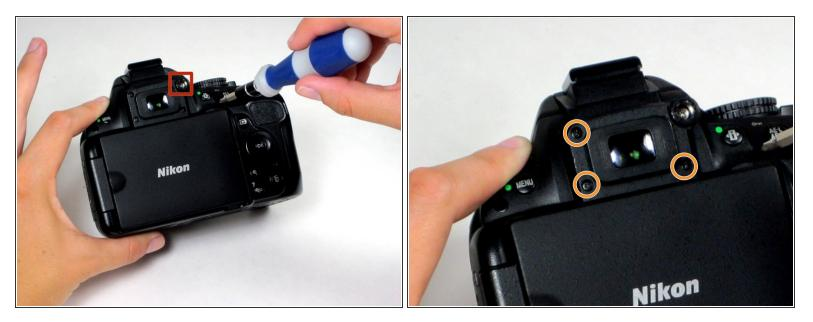
Using a spudger, pry off the diopter adjustment dial cover and remove the screw underneath.
