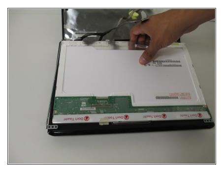
Simply lift the screen from back of the laptop to remove it
