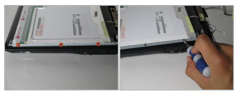
Remove the six 2.0 mm Phillips #1 screws securing the hinges to the screen. There are three screws on each side of the laptop.
