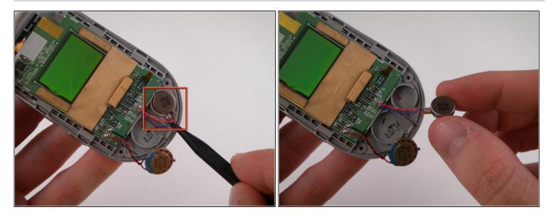
Remove vibrator using the Spudger.
