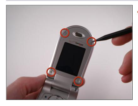
Remove 4 rubber grommets using the Spudger.
