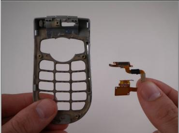
Remove cable from bottom section.
