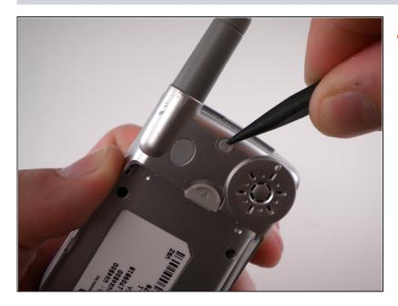
Remove the rubber grommet using a Spudger.
