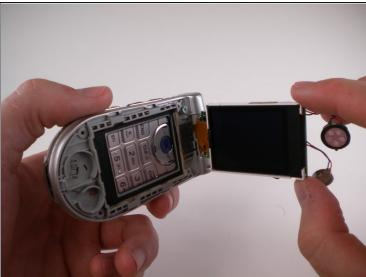
Lift up LCD display using iPod Opening Tool.
