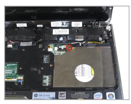
Use the Phillips #1 Screw Driver to unscrew the 5mm screw.
