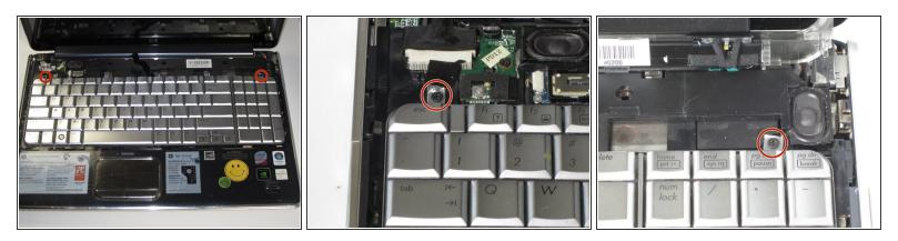
Locate and remove the two 4mm screws with the Phillips #1 screw driver.
