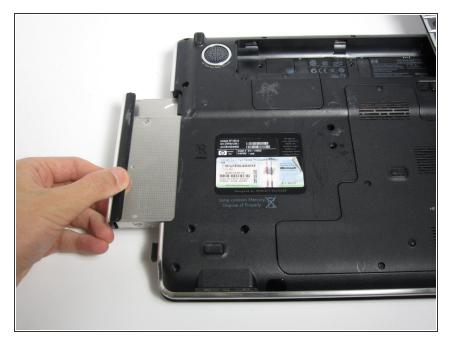
• Push down and pull out the DVD on the left side of the device.
