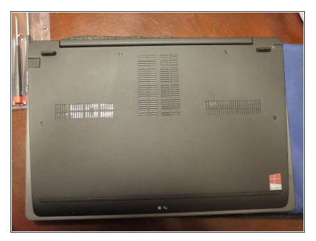
First remove the screws on the bottom of the laptop.
