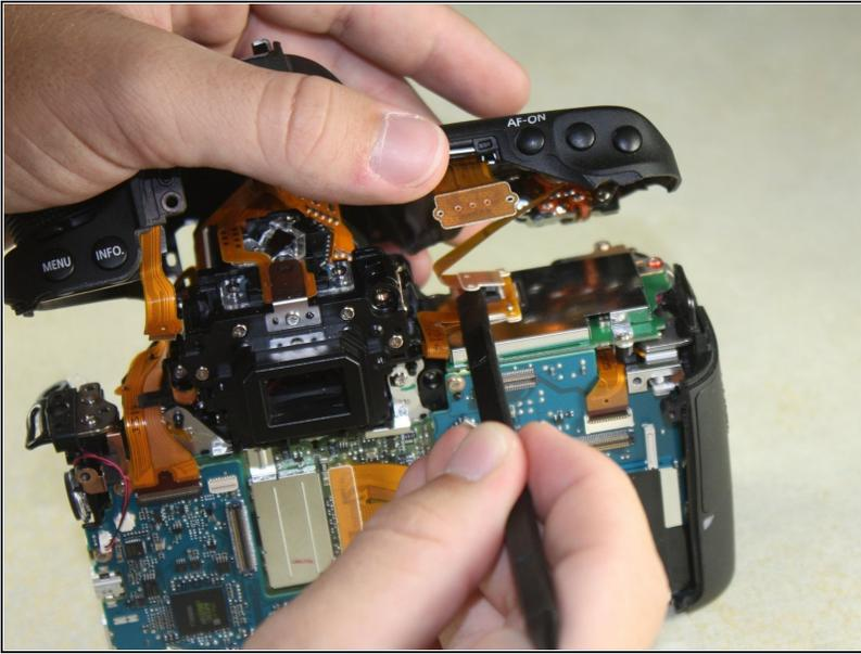
⚠ A ribbon wire connects the inside of the top panel to the body of the camera.
