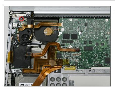
Remove the single Phillips screw from the Bluetooth board.
