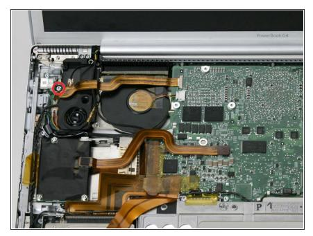
Remove the single T8 Torx screw from the left speaker assembly.
