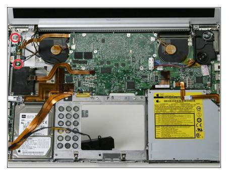
Remove the two identical T8 Torx screws from the DC-In board.
