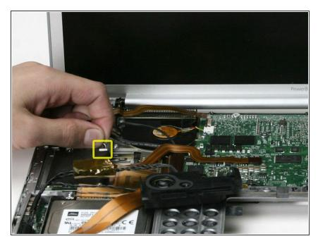
Disconnect the black and white RJ-11 cable from the top, right corner of the modem.
