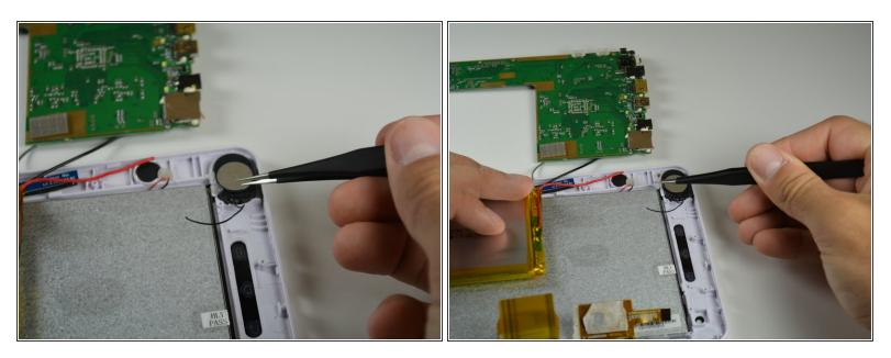
• Remove any hot glue residue holding the speaker in place by peeling it off using tweezers.
