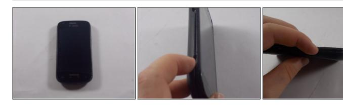
Start by removing the back plastic cover by lifting it up from the notch on the left side of the phone
