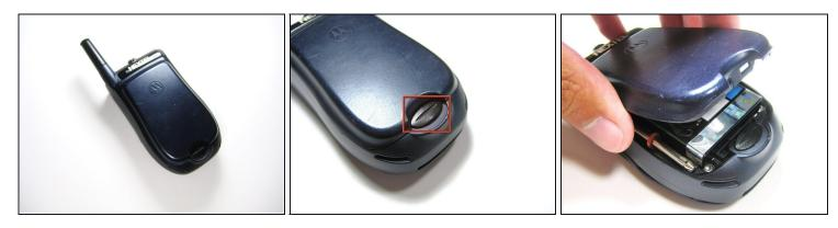
Slide the notch downward while pulling the back cover off to remove it.
