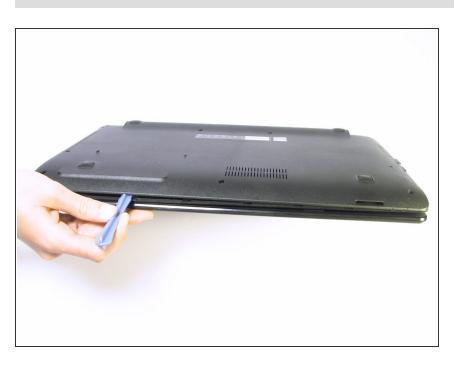
Use the plastic opening tool to separate the keyboard plate cover from the bottom cover. In order to do this, insert the plastic opening tool in between the keyboard plate cover and the bottom cover, then slide along edges to pry open.
