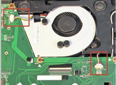
Now, locate the two wires connected to the motherboard.
