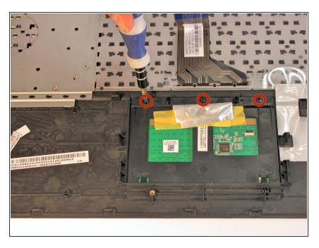
Locate and unscrew the three 3.2 mm Phillips #0 screws at the top edge of the touch pad using the Phillips #0 screwdriver.
