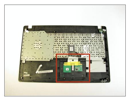
Flip over the keyboard plate cover so the keys are facing down to locate the back of the touch pad.
