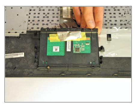
Lift the top edge and gently slide the bottom edge out from underneath the keyboard plate cover.
