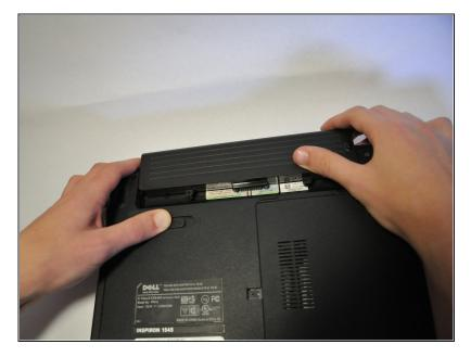
• Slide the release latch while simultaneously pulling backwards on the battery.
