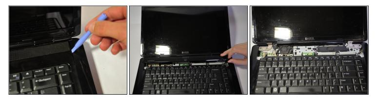
The Center Control Cover is VERY fragile, be careful when using prying tools.
