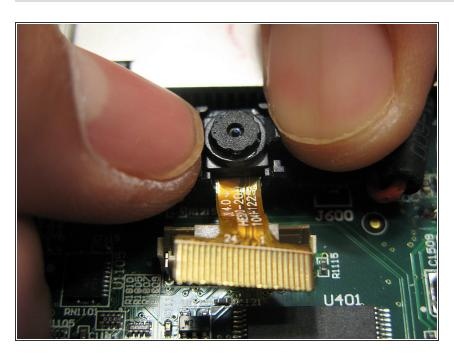
Gently remove the back camera from your motherboard by pushing the black casing away from the camera.
