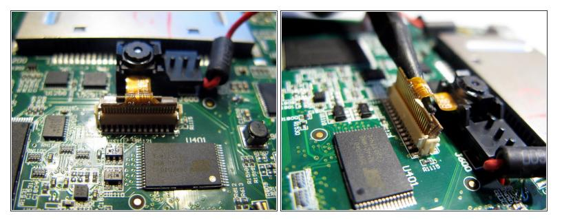
Pull up using a thin plastic tool to disconnect the ribbon connecting the camera to the motherboard.
