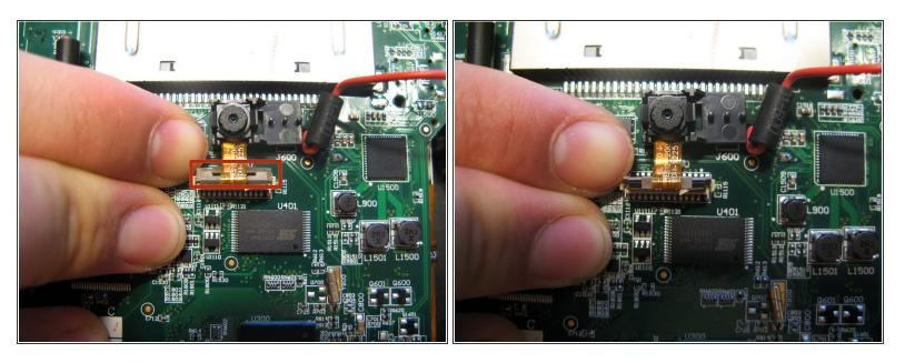
To safely remove the ribbon cable, first you must pull up the retaining flap.
