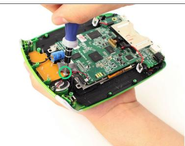
Unscrew the white plastic piece to expose the third 7.0 mm Phillips screw mentioned.
