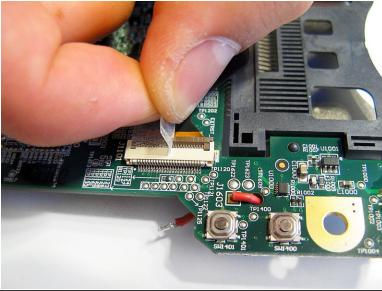
Peel off tape covering the camera's connection ribbon to the circuit.
