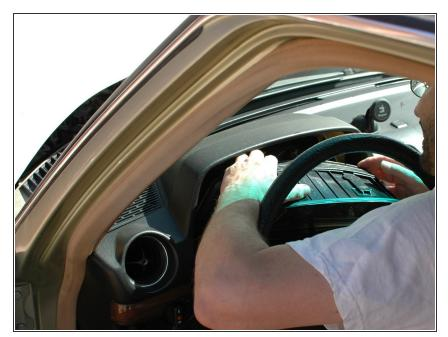
• With everything disconnected you can now remove the cluster, carefully working it up and out past the steering wheel.
