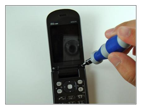
Remove the screws using a Y0 screwdriver.
