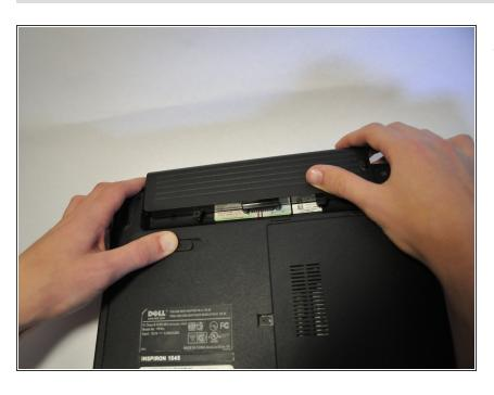
Slide the release latch while simultaneously pulling backwards on the battery.
