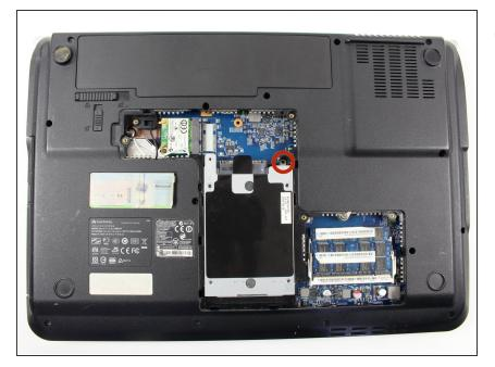
Remove the 1/4" Phillip screw located at the top right of the Hard Drive using a Phillips #0 Screwdriver
