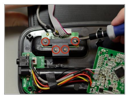
Remove the four 7 mm screws that hold the PCB in place; you will need a Phillips #1 driver to do this. You may need to move some wires out of the way to access one of these screws.
