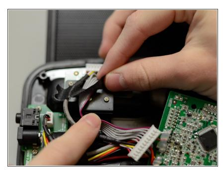
A strip of black tape covers the grey and purple wire cluster that connects to the internal audio printed circuit board. Carefully peel this tape away.
