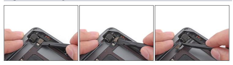
• Use the flat end of a spudger to disconnect the rear-facing camera connector from the logic board.
