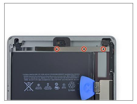
Remove the three 1.4 mm Phillips #000 screws securing the upper component cable bracket.
