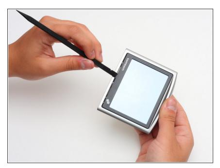
Once separated, use the spudger to pry around the edges of the outer casing.
