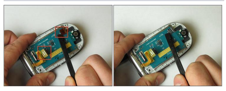
• Unclip circuit attachments located on back of screen circuit board using a Spudger.
