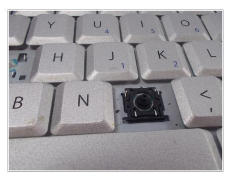
To insert new key, place it directly centered over the rubber nipple and press down firmly.
