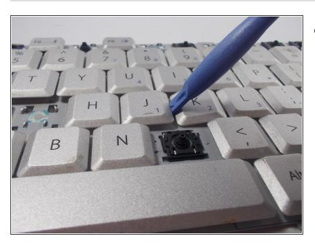
Insert plasitic opening tool into the side of key as shown.
