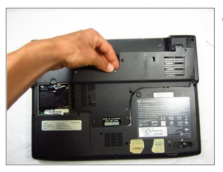
• Pull upwards on the top of the back cover to remove it.
