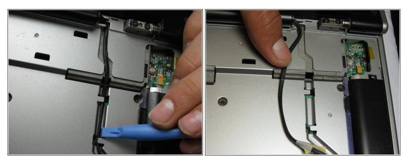
• Use the plastic opening tool to pry out the WiFi cable coming out of the right side of the display from the prongs that hold it in place.
