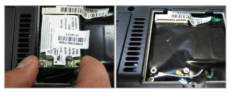
• Hold the WiFi card on both sides and pull outwards to remove it.
