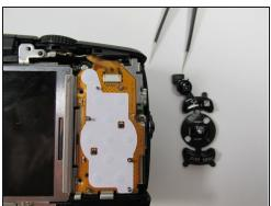
Continue lifting until pad is separated completely from the camera.
