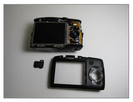
Remove the back cover and the DC IN A/V OUT DIGITAL cover from the camera.
