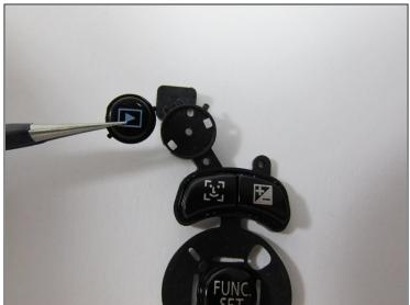
• Once pad is separated from camera, use tweezers to grip button(s) that need to be removed, and lift until it has been separated completely from the pad.
