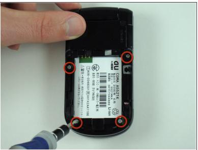
Remove the four screws with the Y0 screwdriver.
