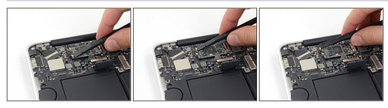
• Use the flat end of a spudger to pry both antenna connectors up from their sockets on the AirPort/Bluetooth card, and move them out of the way.
