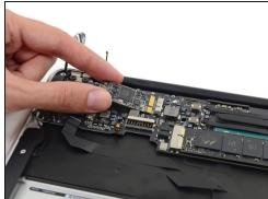
• Slightly lift the free end of the AirPort/Bluetooth board and pull it out of its socket on the logic board.
