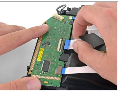
Pull the ribbon cable straight out of the ZIF connector.
