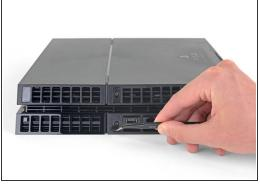
Use tweezers to remove the two stickers in the center of the back of the PS4 exposing two case screws.
