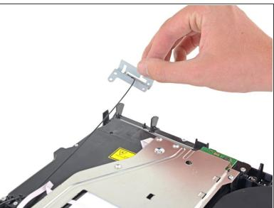
Remove the Wi-Fi antenna.
