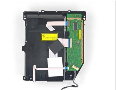
Remove the 6.4 mm Phillips screw from the PCB board.
