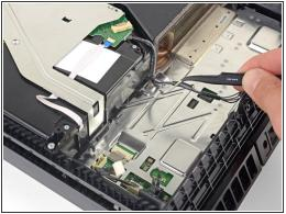
Use your fingers or a pair of tweezers to remove the optical drive cable from the cable guides that hold it in place.
