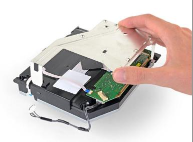
Lift the metal bracket straight up to separate it from the optical drive.
