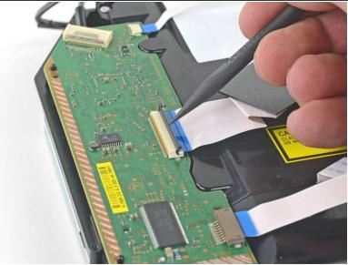
• Use the tip of a spudger to flip open the ZIF connector locking bar.
