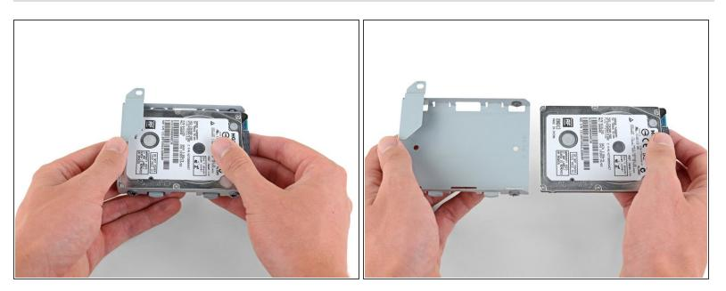
• Remove the hard drive from the hard drive tray.
