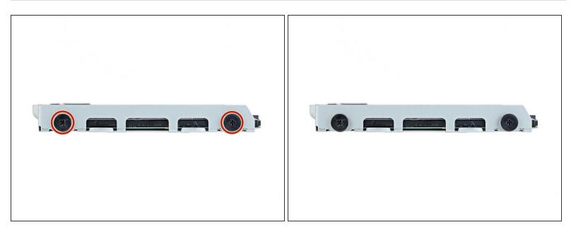
• Remove the two 7.2 mm screws from the right side of the hard drive tray.
