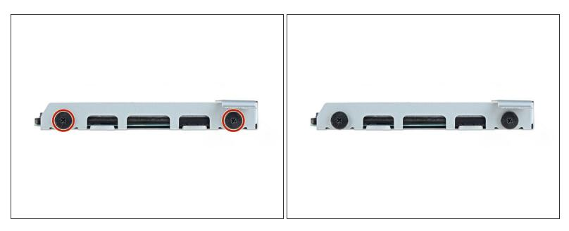
• Remove the two 7.2 mm screws from the left side of the hard drive tray.
