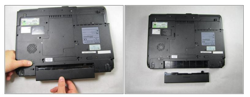
• Hold the release switch and pull out the battery towards you.
