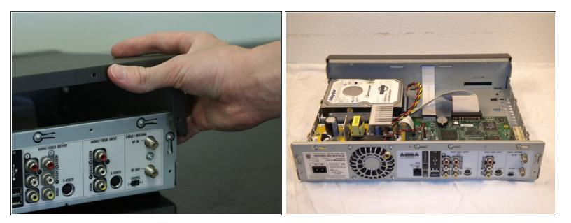
• Lift up and pull back the outer casing towards the rear of the unit.
