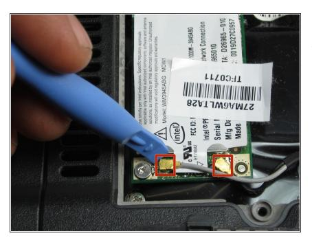
Use the plastic opening tool to gently pry upwards on the two connecting cables to remove them.
