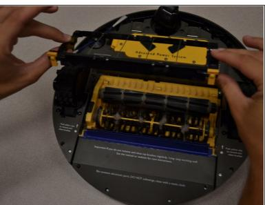
After the guard hinges up, lift the guard up and away from the Roomba.
