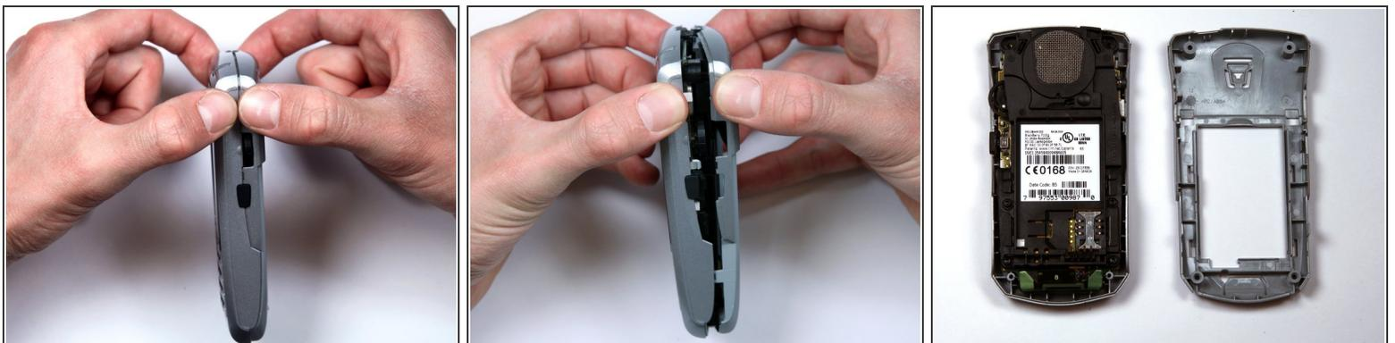
**i** The keypad cover may fall out of the housing when prying the housing apart.
