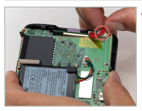
Lift up the circuit board and disconnect the GPS wire, pulling horizontally from its connector port.
