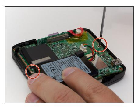
Remove the two screws on that are located on opposite sides of the board.
