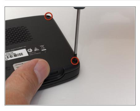
Remove the four screws holding the cover in place by using the Phillips #00 screwdriver.
