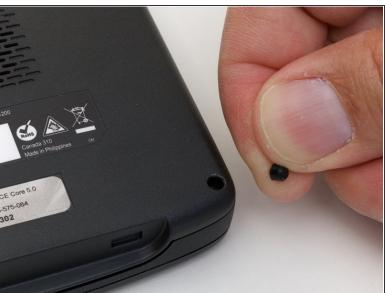
Remove the four rubber caps from the back by using the Phillips #00 screwdriver.
