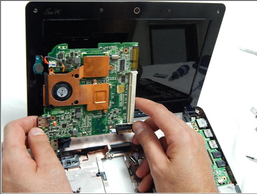
**⚠** Gently lift the motherboard and hold it so that the bottom of the board is exposed.
