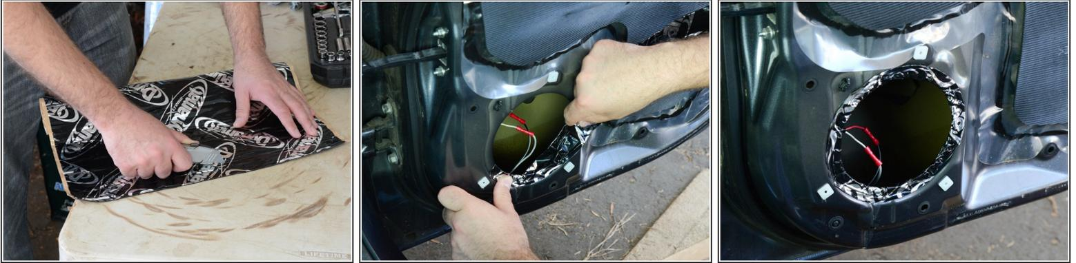
**i** This step is completely optional. Adding a sound deadener like [Dynamat](#) will provide a better seal around the speaker.
