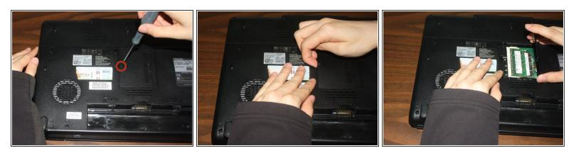
Unscrew the RAM cover and rotate the cover up to remove it. The screw should not be fully removed from the cover itself.
