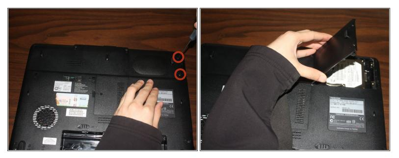
Unscrew the screws enough to remove the top cover.
