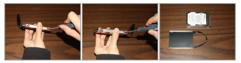
• To separate the hard drive from the caddy, unscrew the two screws.
