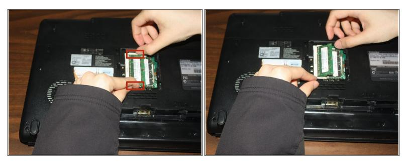
Push the small levers at the sides of the RAM module away from each other. The RAM module should automatically rotate upwards.
