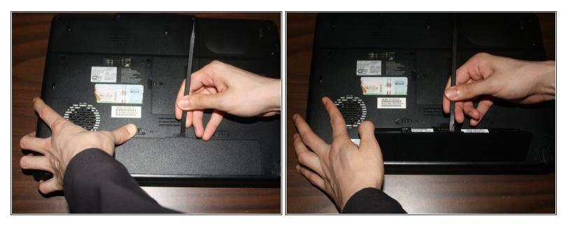
• While holding the left battery lock to the left, lift up the battery using the tab located on the top center of the battery.
