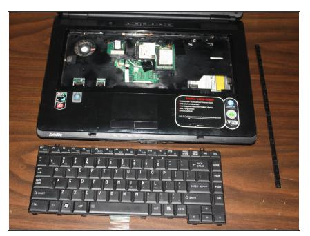
• Remove the keyboard completely from the laptop.
