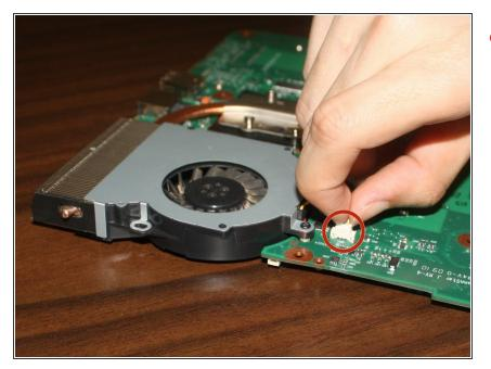
Using your fingers, disconnect the fan power cord from the motherboard.
