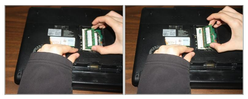
• Remove the RAM module by pulling it out at the angle it was rotated to.
