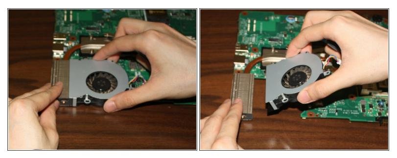
• Using your fingers, disconnect the fan from the heatsink.
