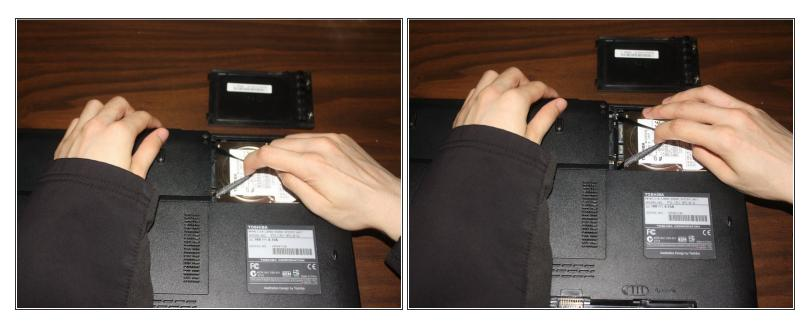
• Remove the hard drive from the SATA slot by tugging lightly on the ribbon cable to the right.
