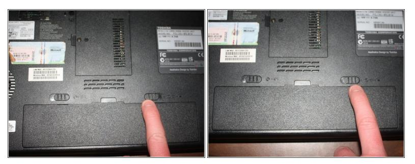
• Locate the right battery lock and slide it to the right.
