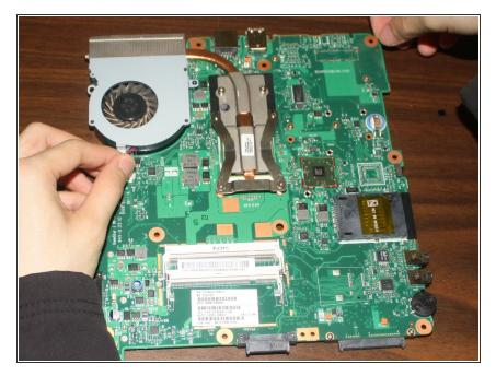
• At this point the motherboard can be fully removed from the laptop.
